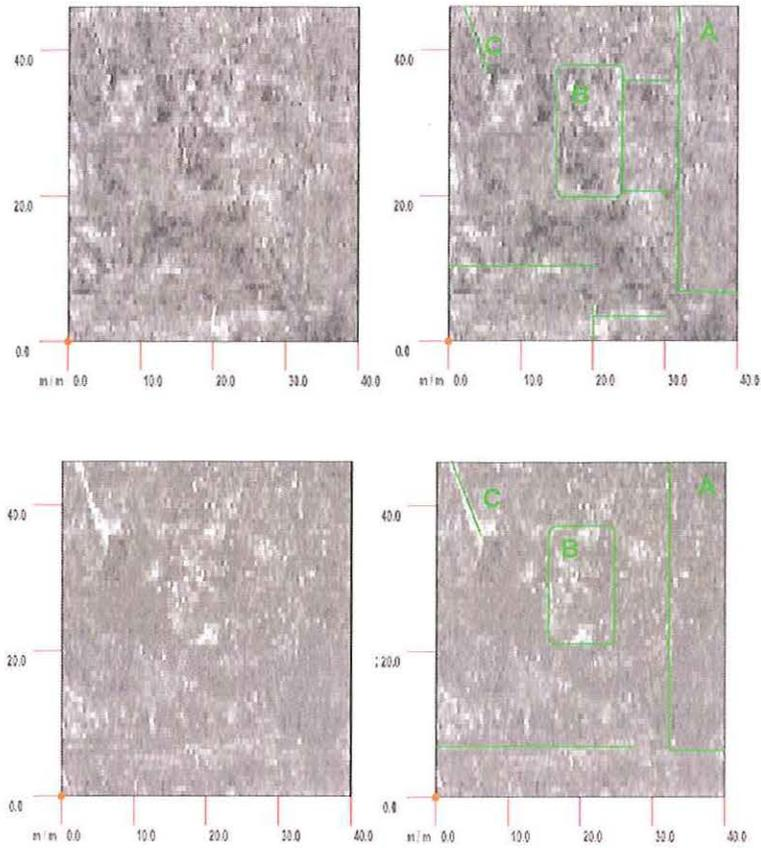
Figure 3. Two sets of time-sliced images from Grid Site 1, Compound A. Horizontal time-slice images for depths of 50 cm (upper plots) and 100 cm (lower plots). The thickness of each slice is 32 cm. In each plot, North is to the left.
