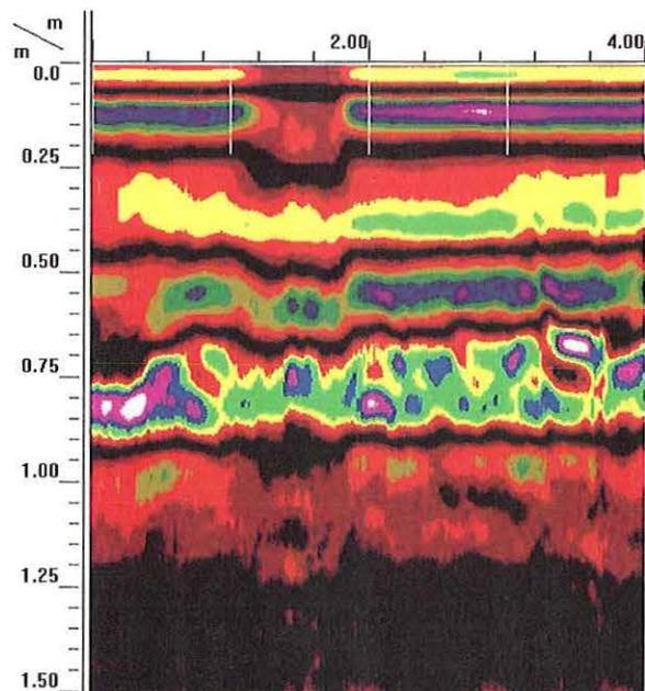
Figure 4. The disruption of surface and near-surface reflections and the faint indentation on this radar record indicates the location of the partially-exposed, buried wall in Grid Site 3.
