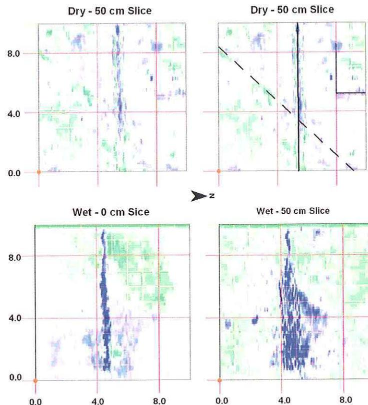
Figure 5. Time-sliced images collected with the 400 MHz antenna from Grid Site 4 (upper plots) under dry conditions and Grid Site 5 (lower plots) under moist conditions.
