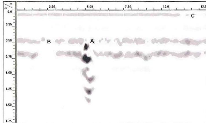
Figure 2. A representative portion of a radar record from Grid 1 (Line X = 40 m) showing both strongly (A) and weakly (B) expressed point reflectors and an area of contrasting surface soil materials (C).
