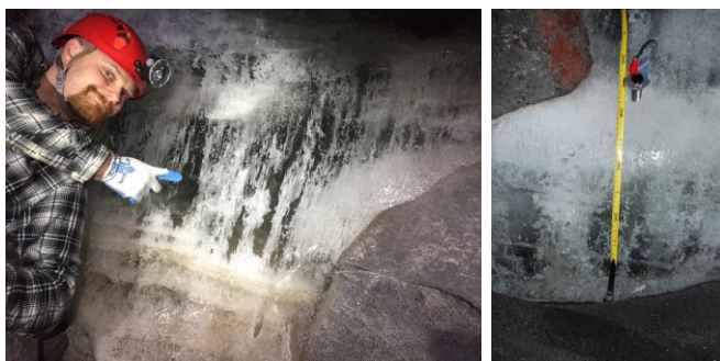
Fig. 3. Left: The ice wall in Cave 455. Right: Recovering short, horizontal ice cores at 2-cm intervals.
